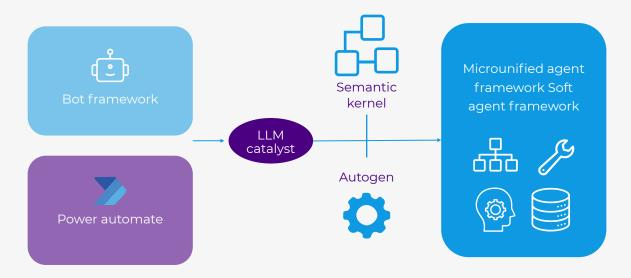
The architectural flow begins with Bot Framework and Power Automate as foundational input layers. These integrate through an LLM catalyst for language-driven orchestration, connecting to Semantic Kernel and AutoGen to enable deterministic and dynamic workflows. The result is the MAF, an adaptive and scalable system that fuses reasoning, tool integration, and memory for next-generation automation.
