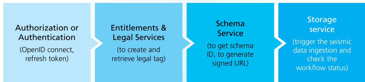
Figure 3: Steps involved in the ingestion of data into the OSDU data platform
