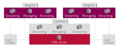
ManageMind CMS / Cloud is an advanced open platform central management station for large installations of up to thousand cameras. The software supports central management of distributed sites, enabling the operator to effectively monitor and manage large video surveillance installations.
