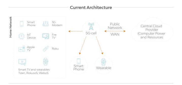
The above architecture will support general applications that do not require low latency. It will not support applications that require low latency such as AR, VR and ML real-time analytics, which will require costly backhaul bandwidth upgrades. Cloudlets will provide the low latency that these applications require by bringing the compute power to the edge and reduce the backhaul costs for the carrier. See the diagram below. We will call this architecture MEC - Media Edge Computing.
