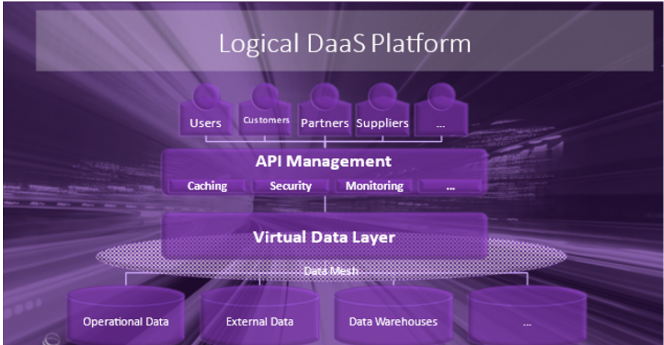
Figure 3. Logical Architecture of a DaaS Platform
