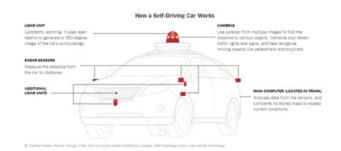
slew of sophisticated LIDAR, RADAR, Cameras and computing units to continuously monitor the surroundings and take split second decisions while driving without human interventions.
